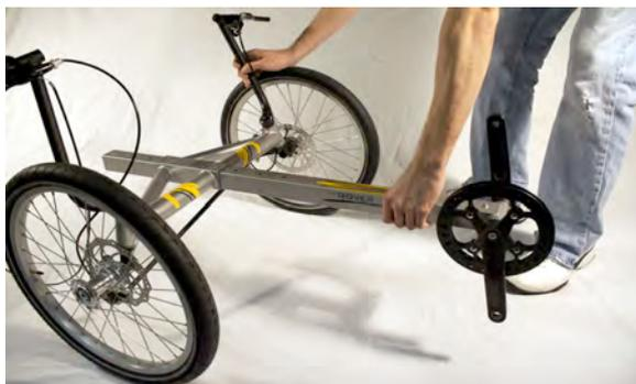
1. Straighten the wheels until they are perpendicular to the front assembly. Insert boom assembly into the “flat” side of the front assembly as pictured (with the chainring on right side of trike).
