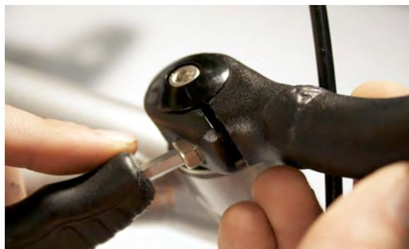
4. Loosen the handlebar fixing bolt on the side of the handlebar and rotate each handlebar so that they extend over the front wheels. You should not have to loosen the top cap bolt to rotate the handlebars.
