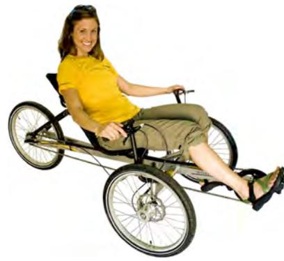
8. Position the seat so that you have about 15 degrees of bend at your knee when the pedal is as far away from you as possible. You do not want your leg to be 100% straight. Tighten the two (upper) bolts that secure the seat clamp to the seat frame.
