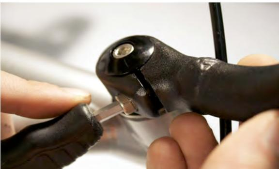
11. Rotate the handlebars to a comfortable position and tighten the handlebar fixing bolts securely. You should not have to adjust the top bolt at all. Double check the tightness of all nuts and bolts and put air in your tires.
