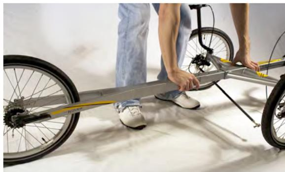
2. Slide rear assembly onto boom with rear cog on right side of trike. The front and rear assemblies should butt up against each other. The holes in the boom are used for sizing the trike to your leg length. The average height rider will have one or two exposed holes in the boom in front of the front assembly (see chart for recommendations).
