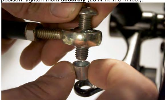
5. **Apply grease** to the bolt and attach the tie rod to the hubmount flange. The tie rod is mounted above the hubmount flange using a 13mm spacer, an M8x40mm bolt and an M8 Nyloc nut on the 8 speed and **below the hubmount flange on the 3 speed**. NEVER allow the chain to ride on the tie rod.
