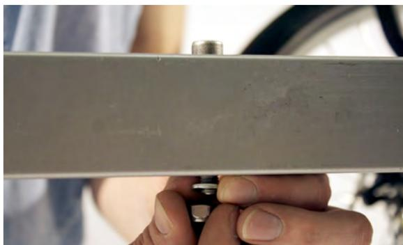
3. **After applying grease** to the four M8x65mm button head socket cap screws, install them with eight M8 flat washers and four M8 Nyloc nuts, but do not tighten at this time. Be sure that all four bolts engage into the through holes in the boom. After you have determined the optimal seating/frame position, tighten them **securely** (20 N-m/175 in-lbs.).
