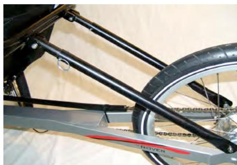
6. **After aligning the front wheels so that they are parallel to each other when pointing straight ahead (neutral toe)**, attach seat assembly to trike: slide the upper seat stay tubes into the lower seat stay tubes and install ring pins. Tighten upper and lower seat stay bolts securely. **Attach shifter cable** to rear hub (see manual) and affix cable to main frame with a zip tie. Secure shifter and brake cables halfway up each handlebar using zip ties.
