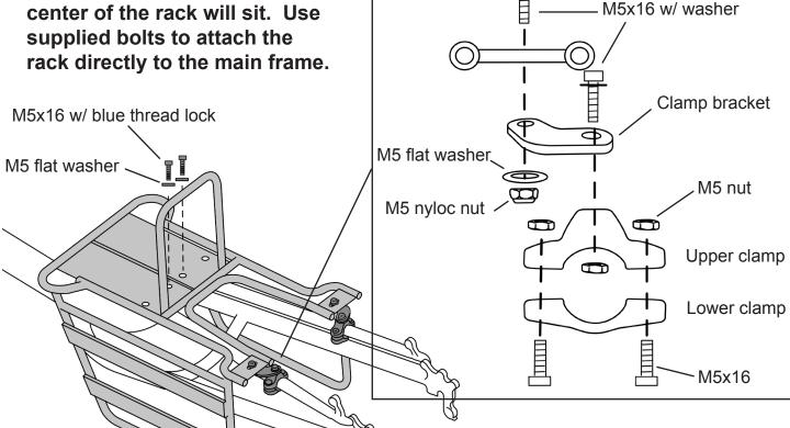
2. Mount Chainstay Clamps as shown. Do not tighten bolts until completely assembled.
