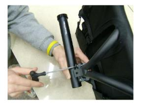
Step four: Attach headrest to the back of the seat with clamp using the four bolts.
