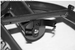
Step 4: Insert the rear fender into the fender support and crimp tabs to secure.
