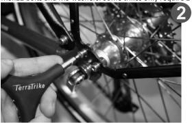
Step 3 (Rover only): Remove rear wheel. Install the rear fender support using the M5x60 bolt, and 50mm spacer.
