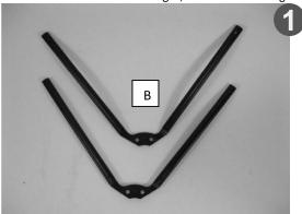
Step 2: Install the assembled fender stays on the trike using 4 M5x12 bolts and M5 washers. Some trikes only require 2 bolts.
