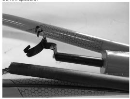
Step 3 (Tandem, Sportster, Tour II only): Remove rear wheel. Install the rear fender support directly to the frame using a M5x12 bolt and washer.
