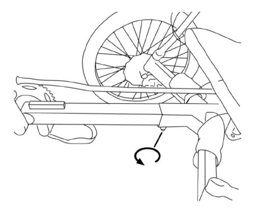
Attach chain and tension with boom.
