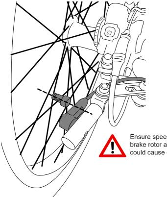
Ensure speed sensor wire is clear of brake rotor and any steering parts that could cause damage. 10
