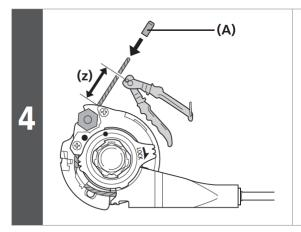
After adjusting the cassette joint, cut off the excess length of inner cable.
