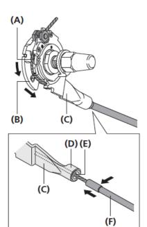
Attach the inner cable to the pulley as shown in the illustration, pass the inner cable through the slit in the bracket, and then insert the end of the outer casing securely into the outer casing holder.
