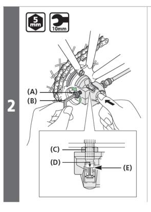
While pushing the bell crank into the hub axle, align the serrations inside the bell crank with the hub nut (C), and continue push until the crank comes into contact with the end face (E) of the hub
