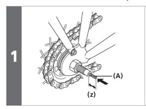
Insert the push rod (A) into the hub axle.
