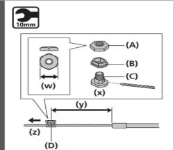
After checking that the end of the outer casing is securely set in the cable adjustment barrel of the REVOSHIFT lever, attach the inner cable mounting bolt unit to the inner cable.
