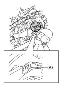
Check that the yellow setting lines on the cassette joint bracket and pulley are aligned with each other.
