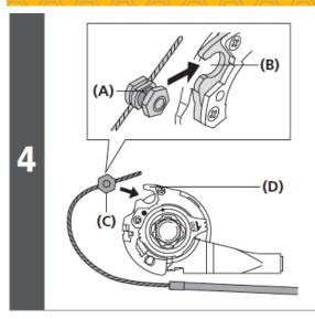
Bring the cable around to the cassette joint pulley, hold it so that the inner cable fixing nut is facing outwards (towards the fork end), and then slide the flats part of the inner cable fixing washer into the gap in the pulley.
